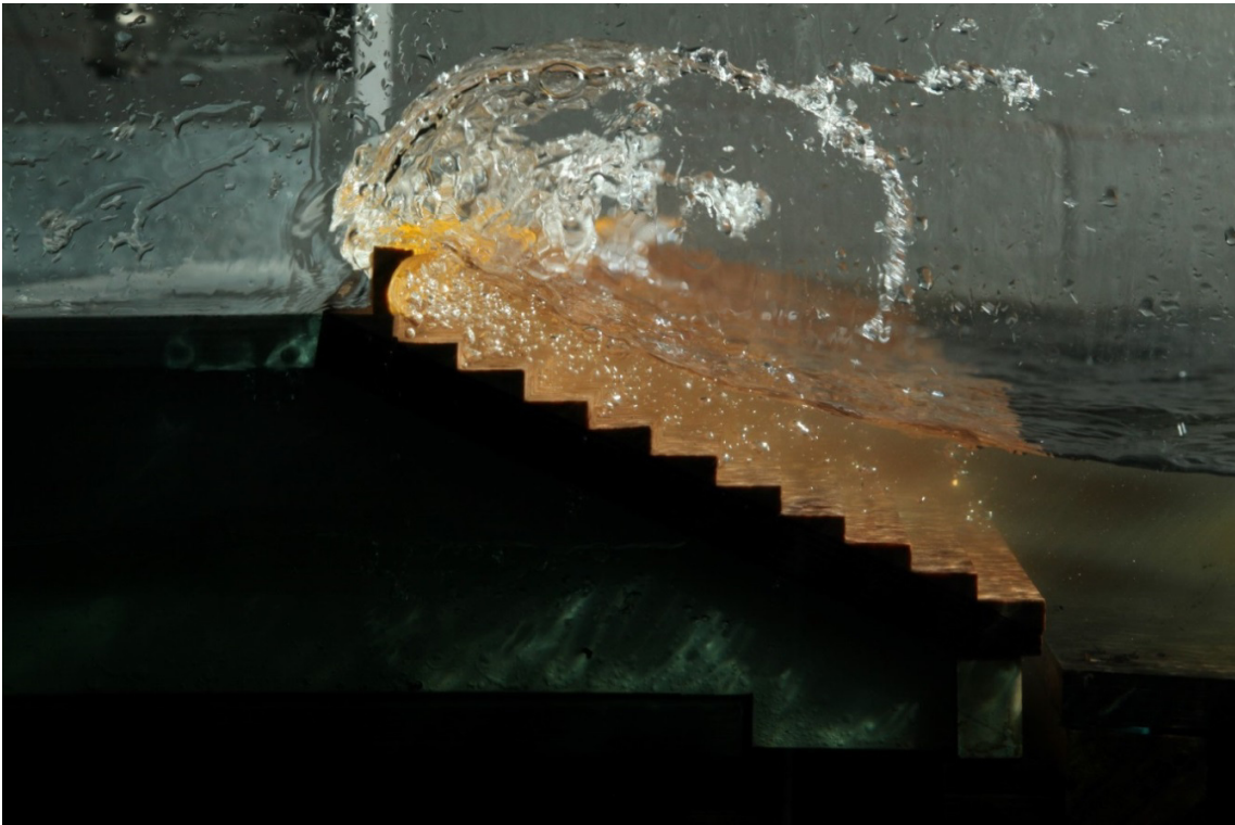
Figure 2: Stepped concrete seawall - Configuration B (6 m AHD Crest, with wave return wall) during 10 year ARI event, present day
